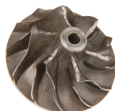
Damage to inducer of turbine wheel
