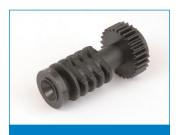
Worm gear failure due to restricted VNT mechanism
