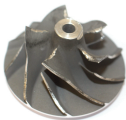
Chipping to the compressor blades
