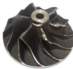
Pitting on the compressor blades
