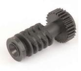
Worm gear failure due to restricted VNT mechanism
