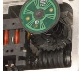
CIPOS gear, worm gear and motor failure. A complete gearbox is required with failures of this nature.
